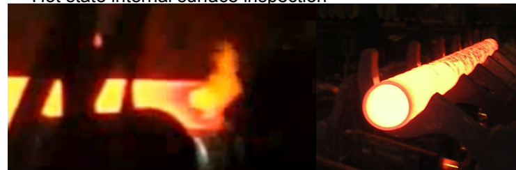
Hot state internal surface inspection
